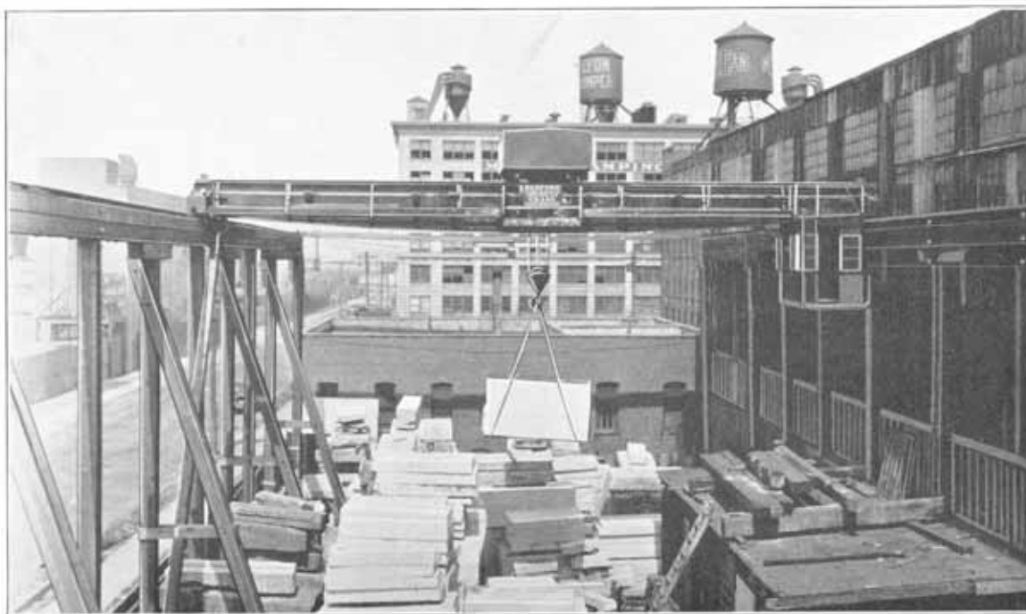
James Gillies & Sons Co., Long Island City, N. Y. 15-ton 52' 0" span three-motor Electric Crane
